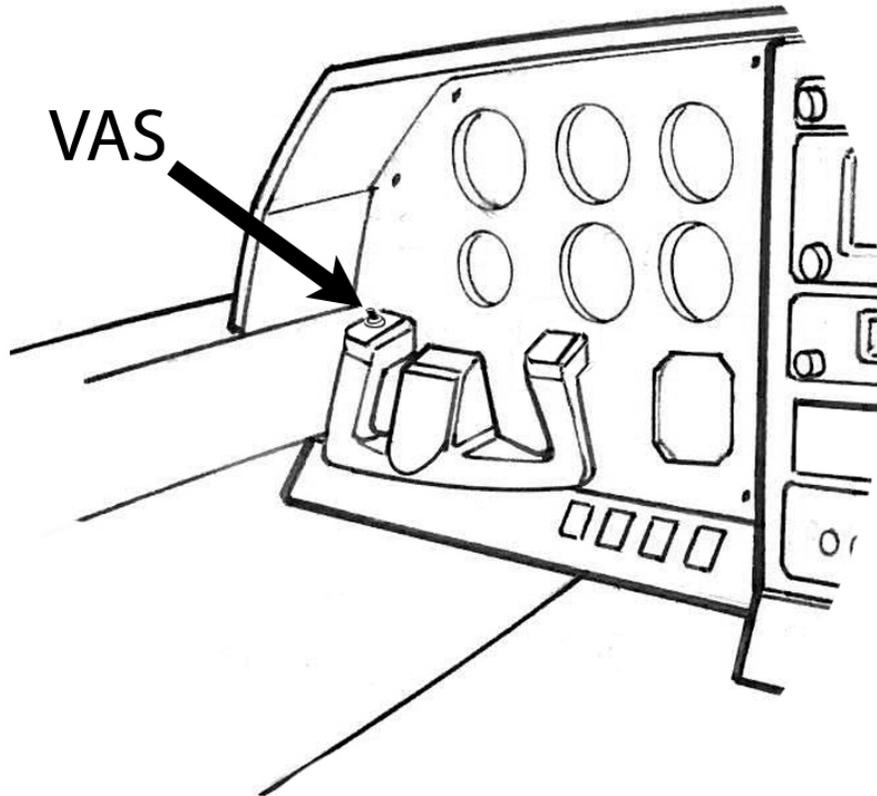
Install VAS so as not to interfere with other yoke switches
