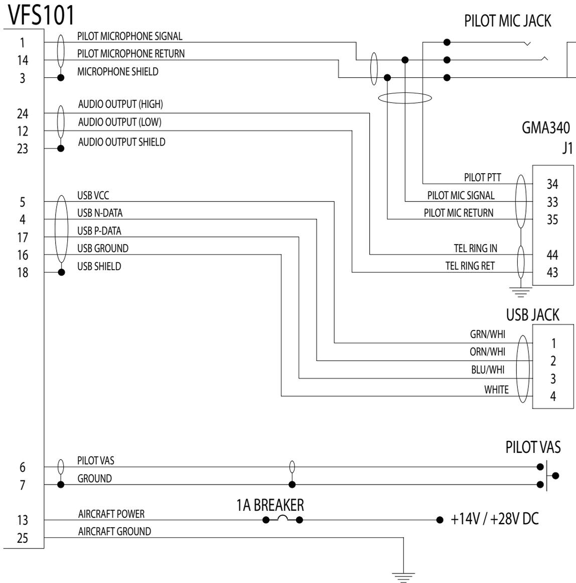
**Note:** VFS101 pin 23 (Audio Output Shield) is internally connected to Aircraft Ground by way of a .1 uF capacitor to prevent ground loops.
